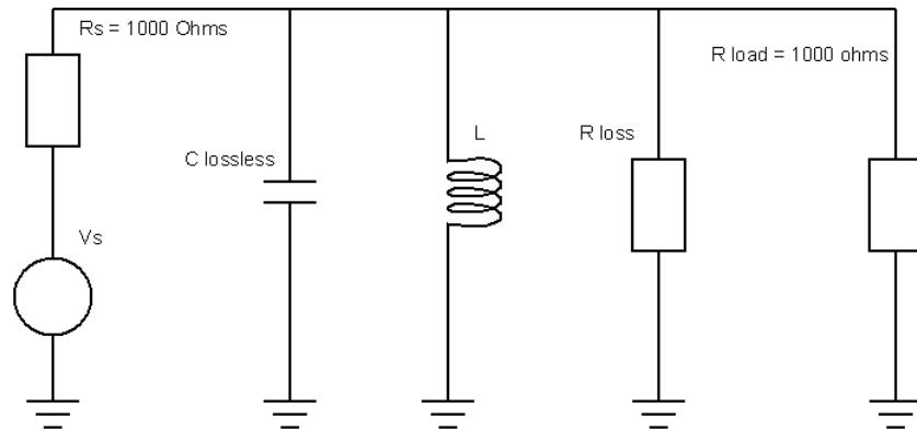
Then, we can replace the equivalent Thevenin voltage source constituted by a pure voltage source  $V_s$  in series with the resistance  $R_s$  by an equivalent Norton current source constituted by a pure current source  $I_s = V_s / R_s$  in parallel with the resistance  $R_s$ .
